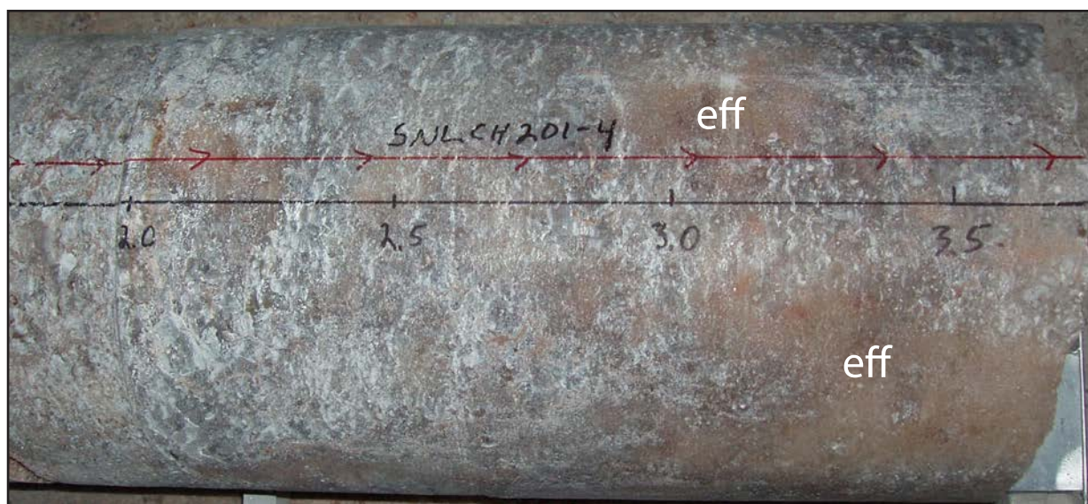
Figure 6. Mixed coarse, gray, translucent halite with fine, light orange to light brown, opaque efflorescent halite (eff) of MU-0. Red and black lines are on the top of the horizontal core. Depth markers are in feet from the rib (wall). Photo courtesy SNL.
